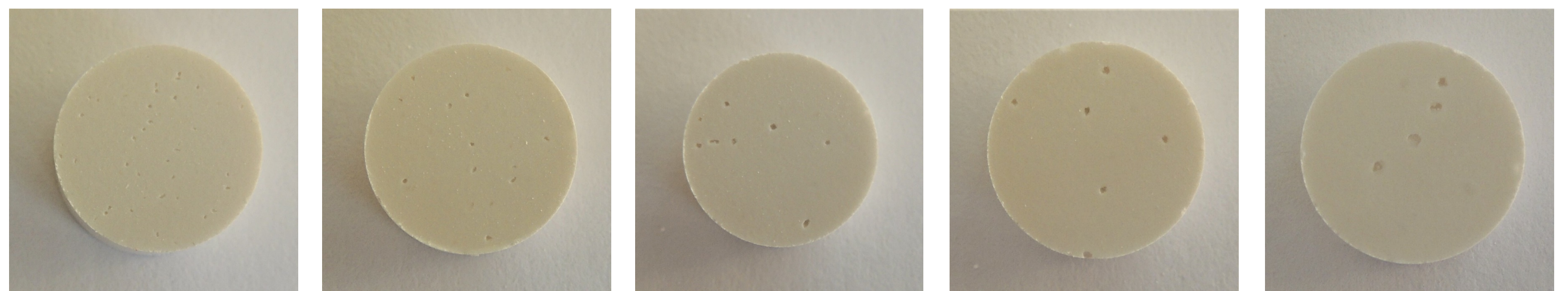
Figure 5: Top view of a heat-treated tablet containing different BHT size fractions. From left to right: fraction 1 to 5.
