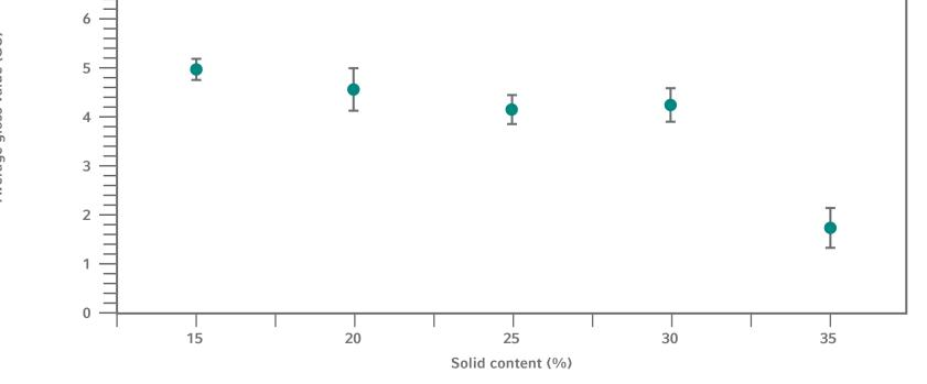
Figure 5: Change of gloss value for (A) AquaPolish® P white 619.03 PRO and (B) AquaPolish® P white 610.38 PRO in dependence of solid content level at elevated tablet bed temperature in the Solidlab 1 batch coater
