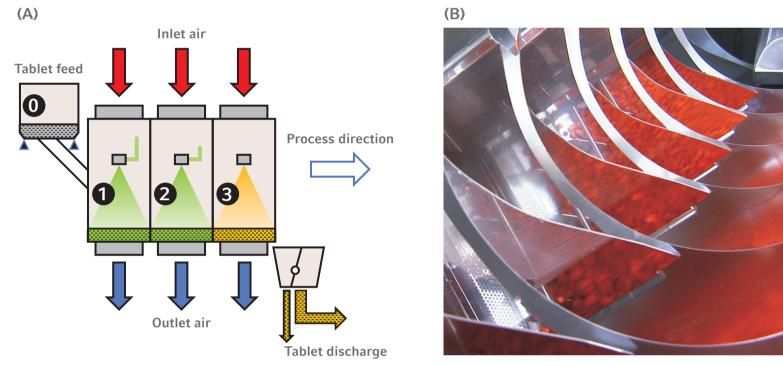
Figure 1: A) schematic presentation of the axial DRN-T 450/3 and (B) view from the outlet through the open front door of DRN-T 1000/7 in transport phase (see flaps in separating walls)
