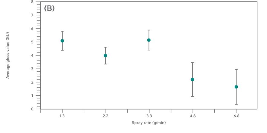
Figure 3: Change of gloss value for AquaPolish<sup>®</sup> P white 619.03 PRO in dependence of (A) different solid content levels and steady spray rate (3.1 g/min) and (B) changing spray rates at 25% solid content in the Solidlab 1 batch coater
