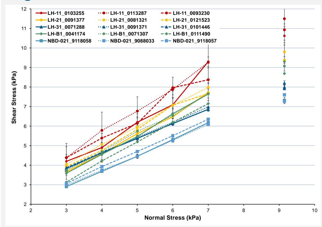
stress shows Shear how easily a previously at rest, consolidated powder will begin to flow; the higher the shear stress for a given normal stress, the less likely the powder will yield and begin to flow if entrapped in a funnel or other vessel under a similar setting stress
