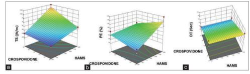
Figure 7: Response surface plot of factorial variable on tensile strength (a) percentage elongation at break (b), and disintegration time (c) for HAMS
