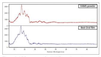
Figure 4: XRD spectrum for HAMS powder and optimized oral film
