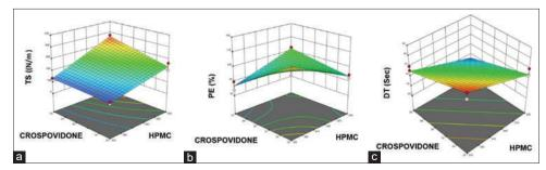
Figure 6: Response surface plot of factorial variable on tensile strength (a), percentage elongation at break (b), and disintegration time (c) for HPMC E 50
