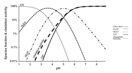
**Figure 3.** Percent fractions of various citric acid (CA) species and their chelation activity calculated at different pH values. The chelation activity (boldly dashed line) is at its maximum above pH 7, when the Cit <sup>3–</sup> concentration is also at its highest. Reprinted with permission from Ref. [37] Copyright 2014, Elsevier.
