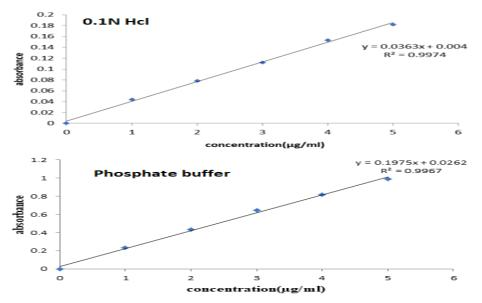
Figure 1: Standard graph of Famotidine in 0.1NHCl and Phosphate buffer
