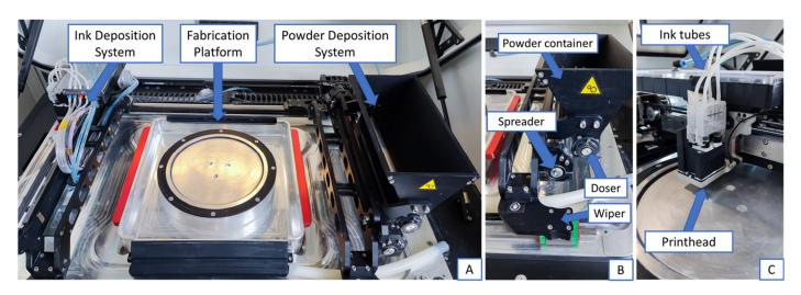
**Figure 1.** Key components of the Picojet D220 3D printer. The main parts are displayed in (**A**), the powder deposition system in (**B**) and the ink deposition system in (**C**).
