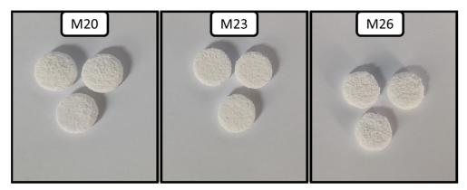
**Figure A1.** Visual representation of 3D-printed tablets from experiments M20 (high strength), M23 (medium strength), and M26 (low strength) with the 20% ethanol-water mixture. As can be discerned, an excess of material at tablet edges is observed for experiment M20, while experiment M26 yielded poorly bonded tablets due to high layer height and low saturation.
