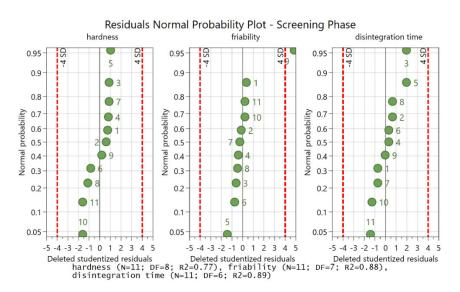
**Figure A2.** Normal probability plot showing the normal distribution of results for hardness, friability, and disintegration time of tablets during the screening phase of the DoE study.
