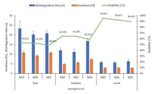
**Figure 6.** Influence of ink composition on disintegration time, hardness, and friability of tablets. Three strength levels of tablets (best, medium, worst) were determined by setting layer height and saturation accordingly. Within each strength level, tablets were prepared with the 10, 20, and 30% ethanol-water mixture.
