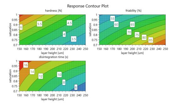
Figure 3. Response contour plot revealing the influence of layer height and the saturation parameter on the mechanical properties of tablets.
