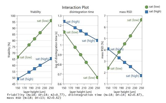
**Figure 4.** Interaction plot between layer height and saturation parameter for friability (left), disintegration time (middle) and mass uniformity (right).
