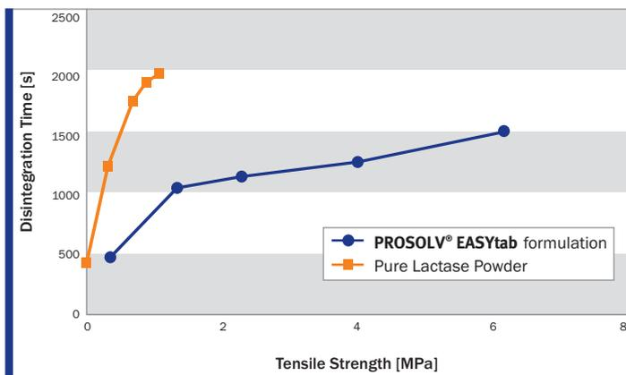
Fig. 5 Comparison of Disintegration Time of Lactase Tablets (200 mg) Composed of either Pure Lactase Powder Containing 1 % Magnesium Stearate as Lubricant or a Blend of Lactase Powder with 30 % of **PROSOLV® EASYtab Nutra CM**.
