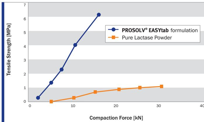
Fig. 4 Comparison of Tensile Strength of Lactase Tablets (200 mg) Composed of either Pure Lactase Powder Containing 1 % Magnesium Stearate as Lubricant or a Blend of Lactase Powder with 30 % of **PROSOLV® EASYtab Nutra CM**.
