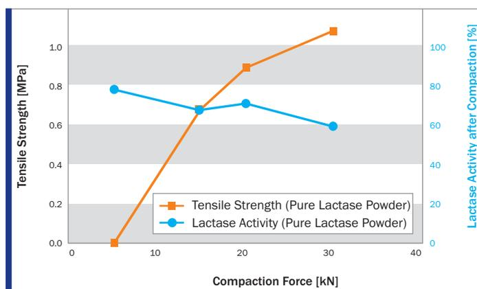
Fig. 3 Effect of Compaction Force on Tensile Strength and Lactase Activity of Tablets of Pure Lactase Powder Containing 1 % Magnesium Stearate as a Lubricant.
