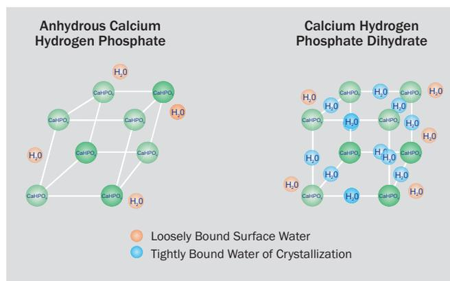
Pic. 4 Surface Water and Water of Crystallization
