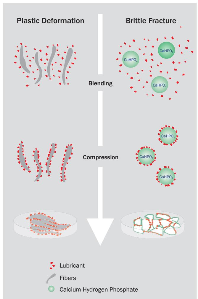
Pic. 2 Reduced Lubricant Sensitivity with **EMCOMPRESS®**. Brittle Fracture Creates Unlubricated Areas for Efficient Binding
