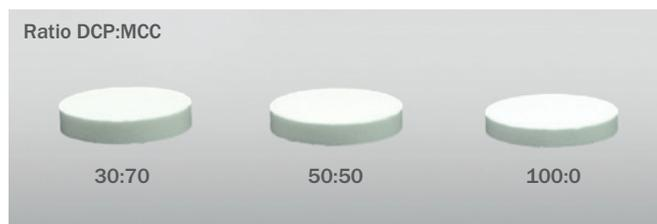
Pic. 3 Effect of Amount of DCP on Tablet Height. Note: All Tablets Have the Same Weight
