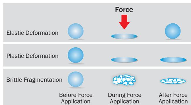
Pic. 1 Deformation Mechanism
