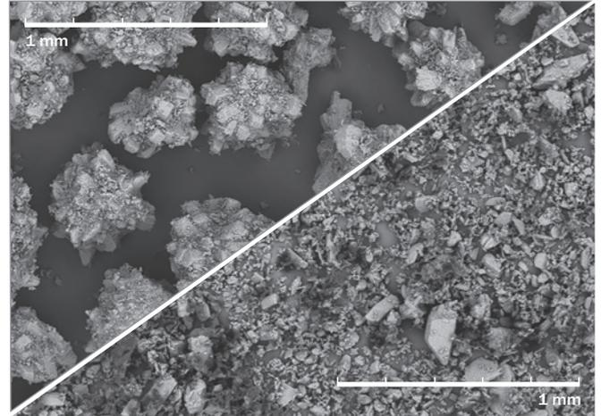
Fig. 1 Micrograph of **EMCOMPRESS® Premium DC / Powder**
