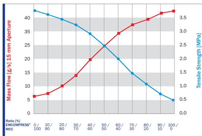
Graph 2 Influence of Different Ratios MCC / **EMCOMPRESS®** on the Mass Flow and the Tensile Strength of Placebo Tablets
