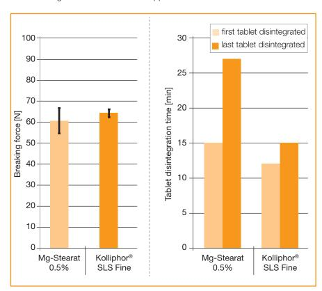
Figure 2: Breaking force and disintegration time of Ibuprofen tablets with Mg stearate compared to Kolliphor SLS Fine.
