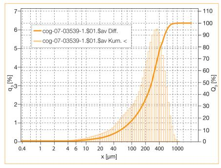
Figure 1: Typical Particle size distribution of Kolliphor SLS Fine measured by laser diffraction.
