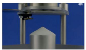
Pic. 5 Excellent Flowability of Members of the  $\mbox{\bf PROSOLV}^{\otimes}$  Family as Shown by the Angle of Repose.
