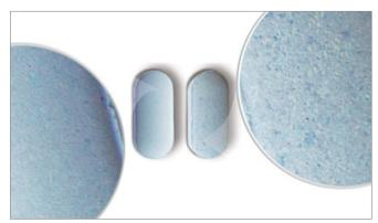
Pic. 6 The Surface Structure Promotes Interactive Blending and, thus, Homogeneous Distribution of Fine-Particle APIs in the Tablet Matrix. The Tablet on the Left was Formulatted with **PROSOLV EASYtab** and a Blue Dye as a Model API. The Formulation Based on Regular MCC (right) Shows a Spotty Appearance Indicating in Homogeneous Distribution of the Model API.
