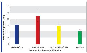
Fig. 1 Surface Roughness of Tablet Cores
