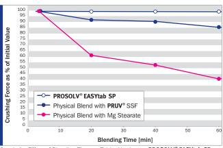
Graph 1 Effect of Blending Time on Tablet Hardness. PROSOLV® EASYtab SP in Comparison with Physical Mixtures of Microcrystalline Cellulose (MCC), Colloidal Anhydrous Silica (CSD), Sodium Starch Glycolate (SSG) and Sodium Stearyl Fumarate (SSF) or Magnesium Stearate, Respectively, as a Lubricant.
