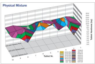
Graph 7 Tablet Hardness Uniformity -\* Physical Mixture with 40 % Paracetamol.
