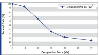
Graph 4 Correlation between Compression Force and Viability of Bacteria Cells in Directly Compressed Probiotic Tablets Containing 20 % of the Bifidobacteria Strain BB-12.
