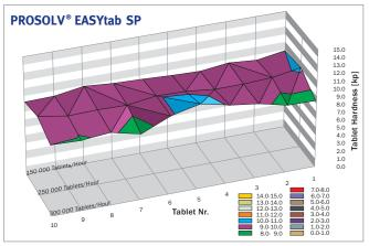
Graph 8 Tablet Hardness Uniformity -\* PROSOLV® EASYtab SP with 40 % Paracetamol.
