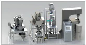
Pic. 12 Continuous Tablet Manufacturing Line. (Courtesy of University of Eastern Finland, Kuopio)
