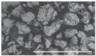
Pic. 4 SEM of **PROSOLV® EASYtab NUTRA** Particle Size and Morphology of the Composite Material Enable Good Powder Flow and High Content Uniformity.
