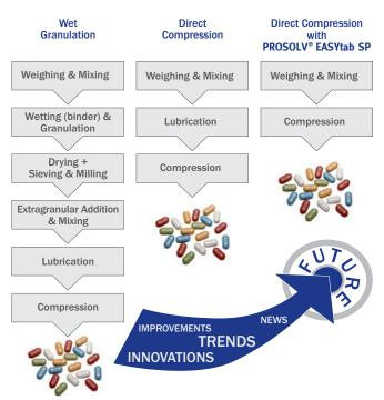
Fig. 1 Comparison of the Number of Production Steps for Different Ways of Manufacturing Tablets.
