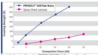
Graph 5 Crushing Strength of **PROSOLV® EASYtab Nutra** and Spray-Dried Lactose at Different Compaction Forces.
