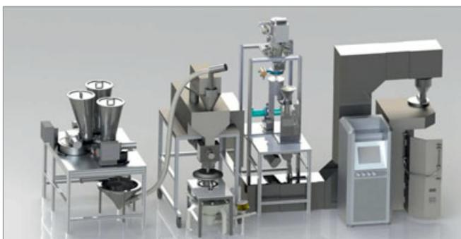
Pic. 12 Continuous Tablet Manufacturing Line.
