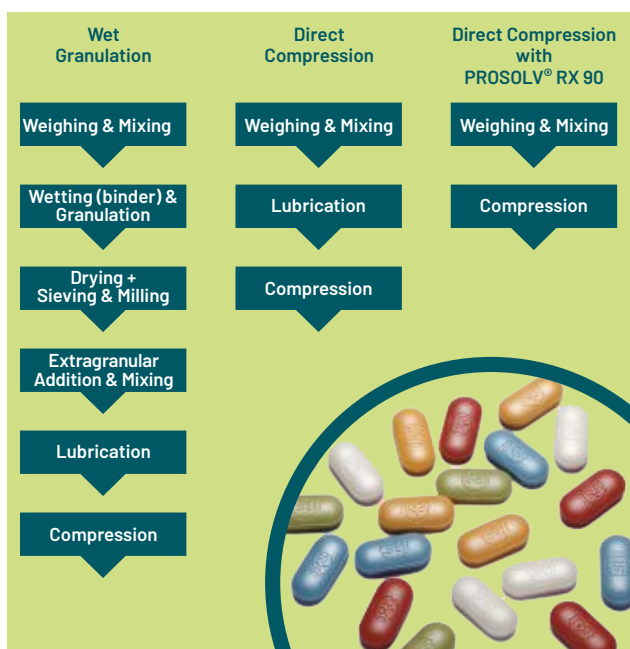
Fig. 10 Comparison of the number of production steps for different ways of manufacturing tablets
