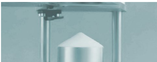
Pic. 5 Excellent flowability of members of the PROSOLV® Family as shown by the angle of repose.
