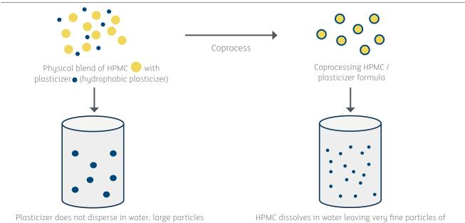
Plasticizer does not disperse in water; large particles will not pass through spray nozzle or form film HPMC dissolves in water leaving very fine particles of plasticizer in suspension. Fine particles will flow through the spray nozzle and form a smooth, slick film
