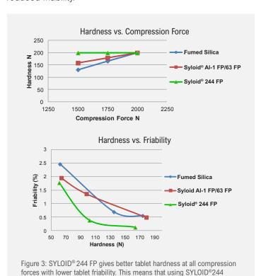
FP allows compression at lower forces while still delivering good tablet
