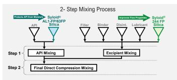
Figure 2: SYLOID® FP Silicas can be used in both steps of a 2-step mixing process. SYLOID® 244 FP silica is used as a glidant in the excipient part of the formulation. It has the capacity to take up excessive moisture from the other excipients while maintaining plasticizing properties. SYLOID® AL-1 FP/63 FP silica, which is effective for moisture control of sensitive molecules, is mixed with the active ingredients to absorb moisture and provide maximum stability to the formulation mix.
