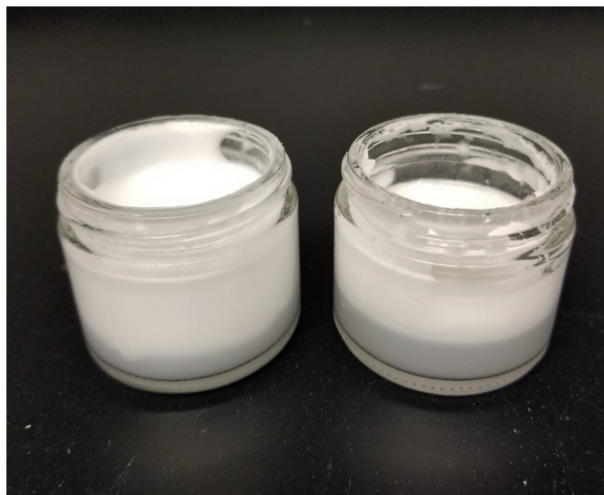
Phase Separation of Two Creams: When emulsion oil droplets coalesce into larger droplets, they migrate upwards causing the underlying layer to appear darker. This is called “creaming.”
