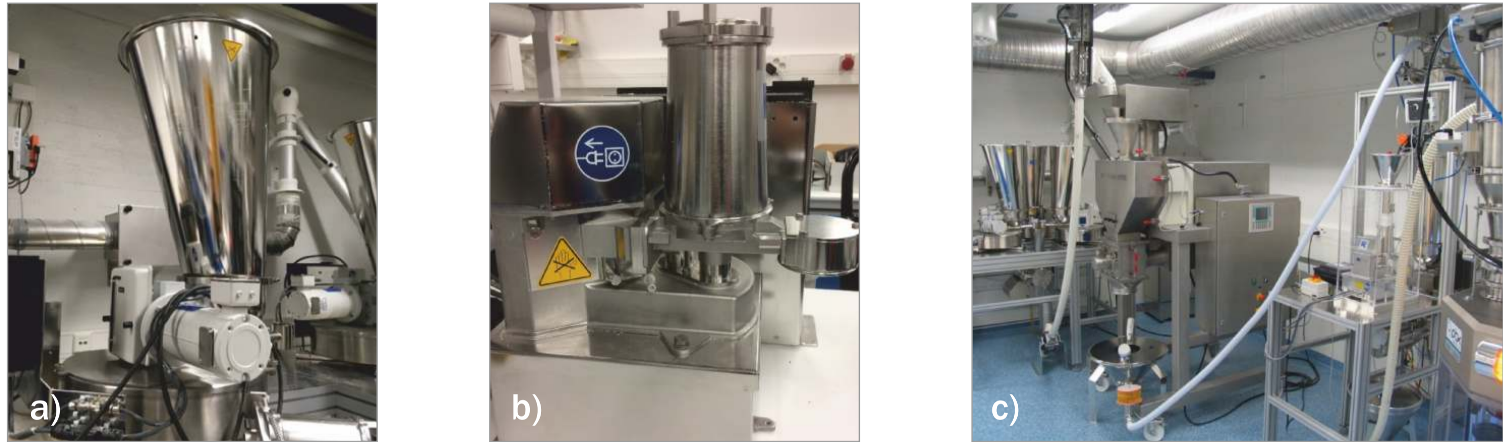
Pic 1 Equipment Used in this Study a) Standard Feeder (Load Capacity ≈ 20kg); b) Microfeeder (Load Capacity 200-300 g); c) Continuous Manufacturing Line
