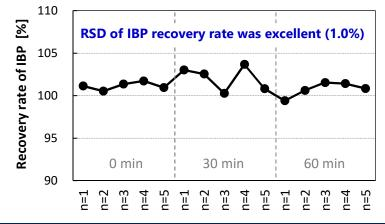
Recovery rate of Ibuprofen (IBP) in each tablet was measured at 0, 30, 60 minutes during tableting by rotary-press.
