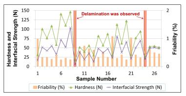
[Figure 5] Interfacial strength and friability of bilayer ODTs containing APIs
