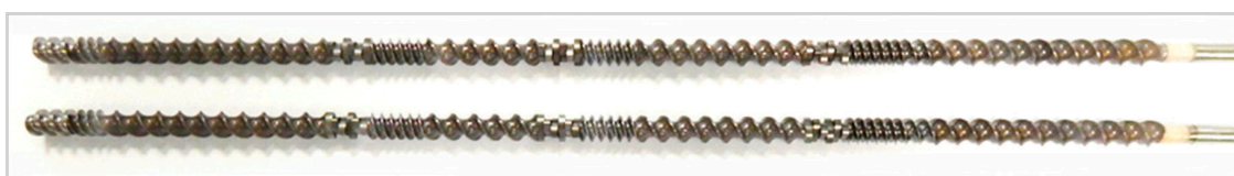
Figure 2. Screw configuration for Thermo Fisher Scientific ® Pharma 11-mm extrusion.
