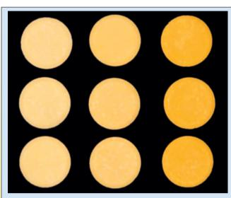
Figure 2: Visual appearance of tablets containing different amounts of riboflavin – formulation #4 (left), #5 (middle) and #6 (right)
