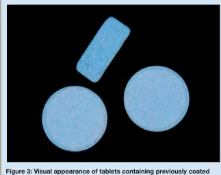
Figure 3: Visual appearance of tablets containing previously coated Ludiflash<sup>®</sup>
