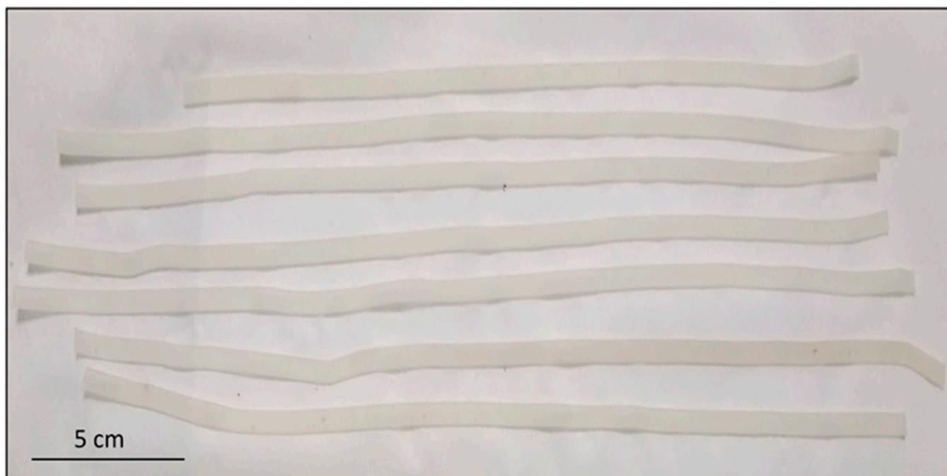
**Figure 1.** Picture showing the extruded stripes of the batch containing 50% wt of API and 5% wt of Guar gum. Scale bar 5 cm.
