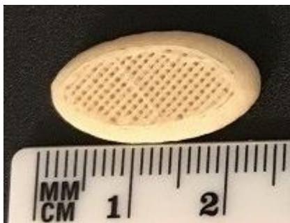
Figure 1: 3D printed tablet with porous core: elliptical shape with dimensions of 22 mm length, 12 mm width and 5 mm height. Infill percentage 47.3%. No top or bottom layer were printed.
