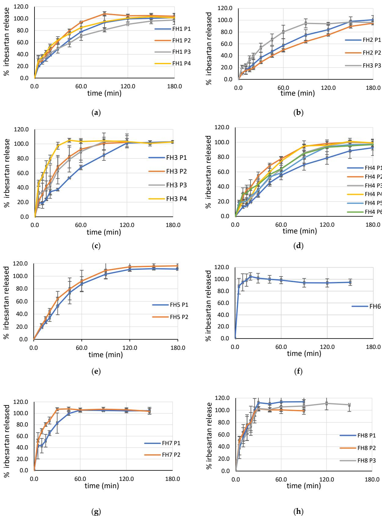
**Figure 9.** Drug release from irbesartan SLS tablets produced with different laser speeds: P1-100.00 mm/s, P2-120.00 mm/s, P3-140.00 mm/s, P4-160.00 mm/s, P5-180.00 mm/s, and P6-220.00 mm/s; (a) FH1, (b) FH2, (c) FH3, (d) FH4, (e) FH5, (f) FH6, (g) FH7, and (h) FH8.
