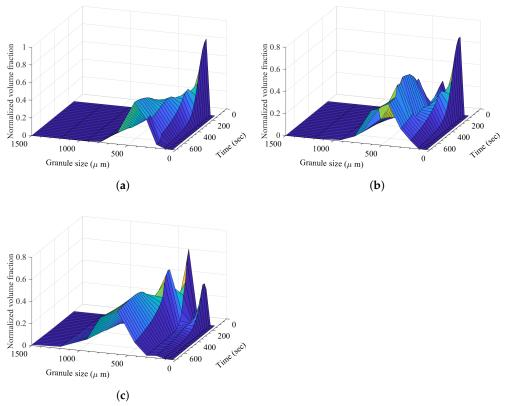
**Figure 13.** Granule size distribution with increase in granulation time at a varying degree of hydrophobic content (ibuprofen). (a) Granule size distribution with increase in granulation time at 40% hydrophobic component (ibuprofen), (b) granule size distribution with increase in granulation time at 50% hydrophobic component (ibuprofen), and (c) granule size distribution with increase in granulation time at 60% hydrophobic component (ibuprofen).
