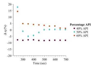
Figure 15. Model predicted granule API content with increase in wet massing time.
