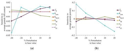
**Figure 7.** Effect of changes in adjustable parameter values on porosity and API content. (**a**) Sensitivity to average API content, (**b**) Sensitivity to granule average porosity
