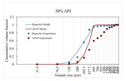
Figure 10. Model validation using 50% API formulation.
