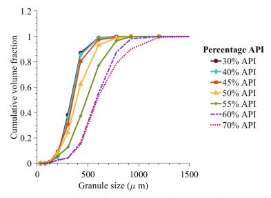
**Figure 12.** Cumulative volume fraction prediction with change in percentage composition of API and 0.6 liquid-to-solid ratio.
