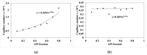
**Figure 4.** Change in capillary numbers with increase in API fraction. (**a**) Ibuprofen and MCC101 formulation, (**b**) Acetaminophen (APAP) and MCC101 formulation.
