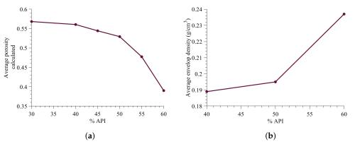
**Figure 16.** Change in granule micro-structure with increase in API content. (**a**) Model predicted average porosity, (**b**) Experimental envelop density.
