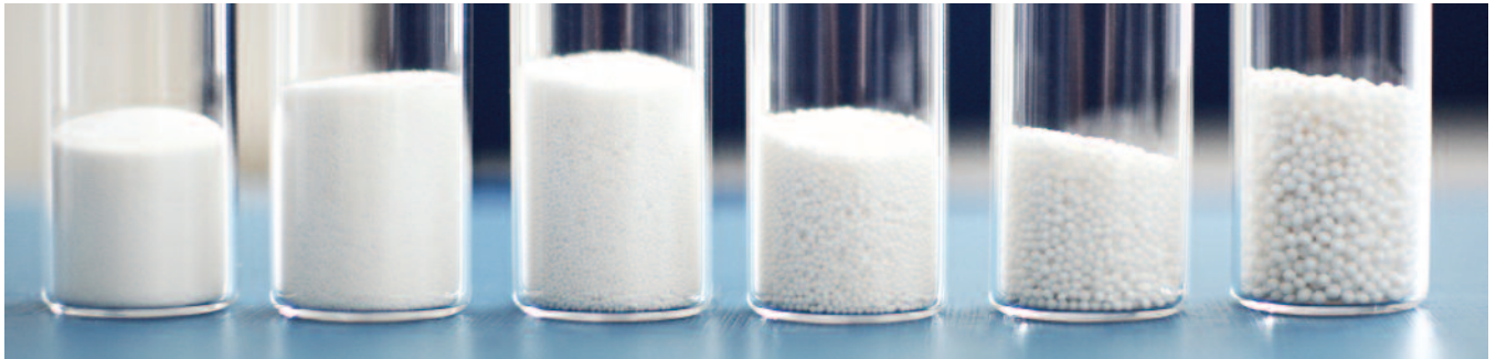
Six size grades of Cellets MCC starter pellets: 100 (100 to 200 microns); 200 (200 to 355 microns); 350 (350 to 500 microns); 500 (500 to 710 microns); 700 (700 to 1,000 microns); and 1000 (1,000 to 1,400 microns).
