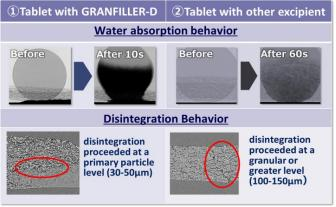
Fig. 3 Image of water absorption and disintegration
