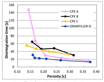
Fig.4 Effect of porosity on disintegration time
