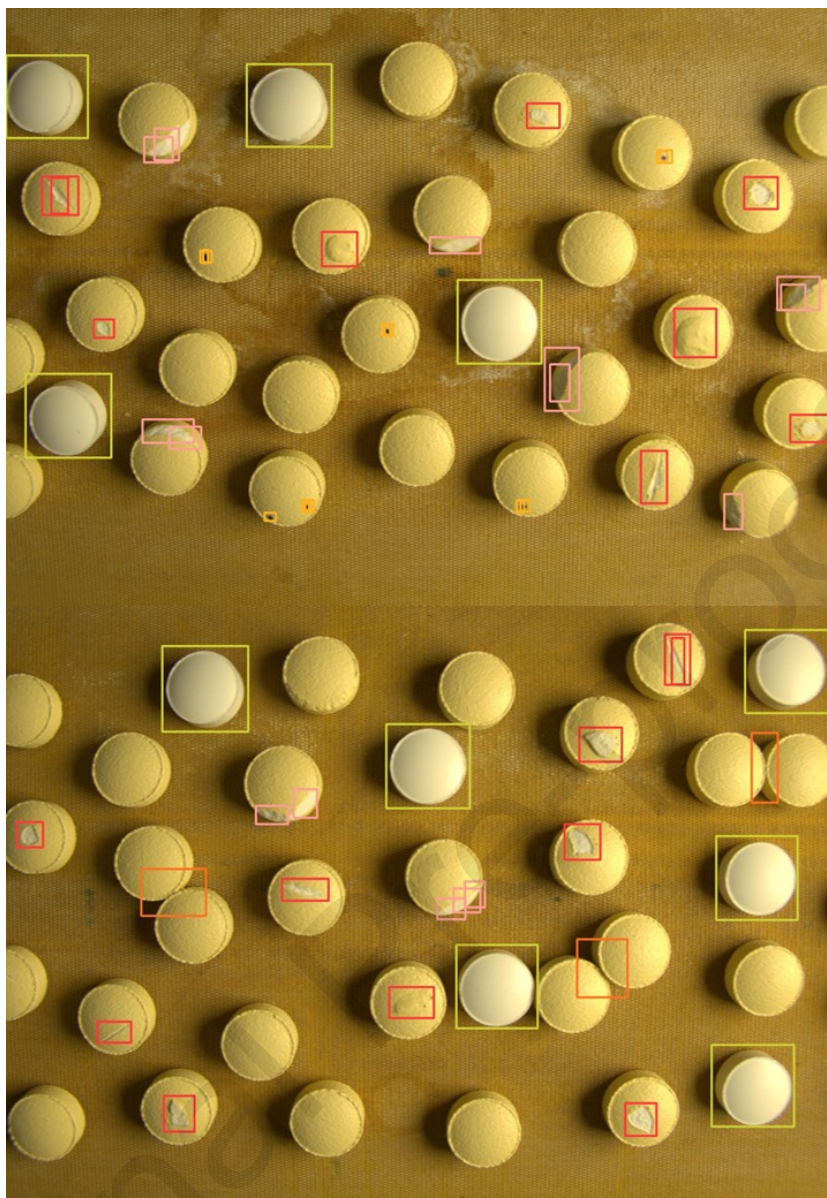
Fig. 4. Two images with classified tablets. Bounding box colouring: yellow: uncoated tablet; light orange: dotted defect; dark orange: twinning tablets; red: uneven surface; pink: edge defect.
