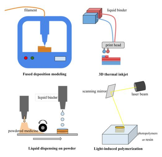
Figure 1. Common 3D printing processes used in pharmaceutical dosage form preparation
