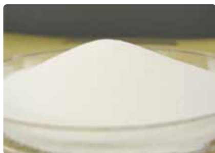
Neusilin® US2 +30% linseed oil, Dry at 50 °C
