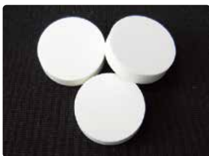
Linseed oil tablet, Ø11.3mm, 125 N at 500 kg/cm 2
