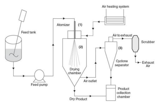
**Figure 3.** Illustration of spray-drying mechanism (1) atomizer; (2) sprayed droplets; (3) product collector [53].
