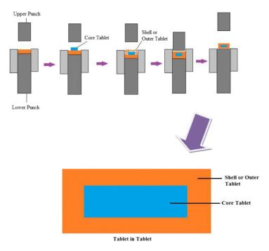
**Figure 2.** Illustration of direct compression coating process [49].
