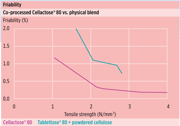
Figure 12: Friability of tablets produced with either Cellactose® 80 or its corresponding physical blend.
