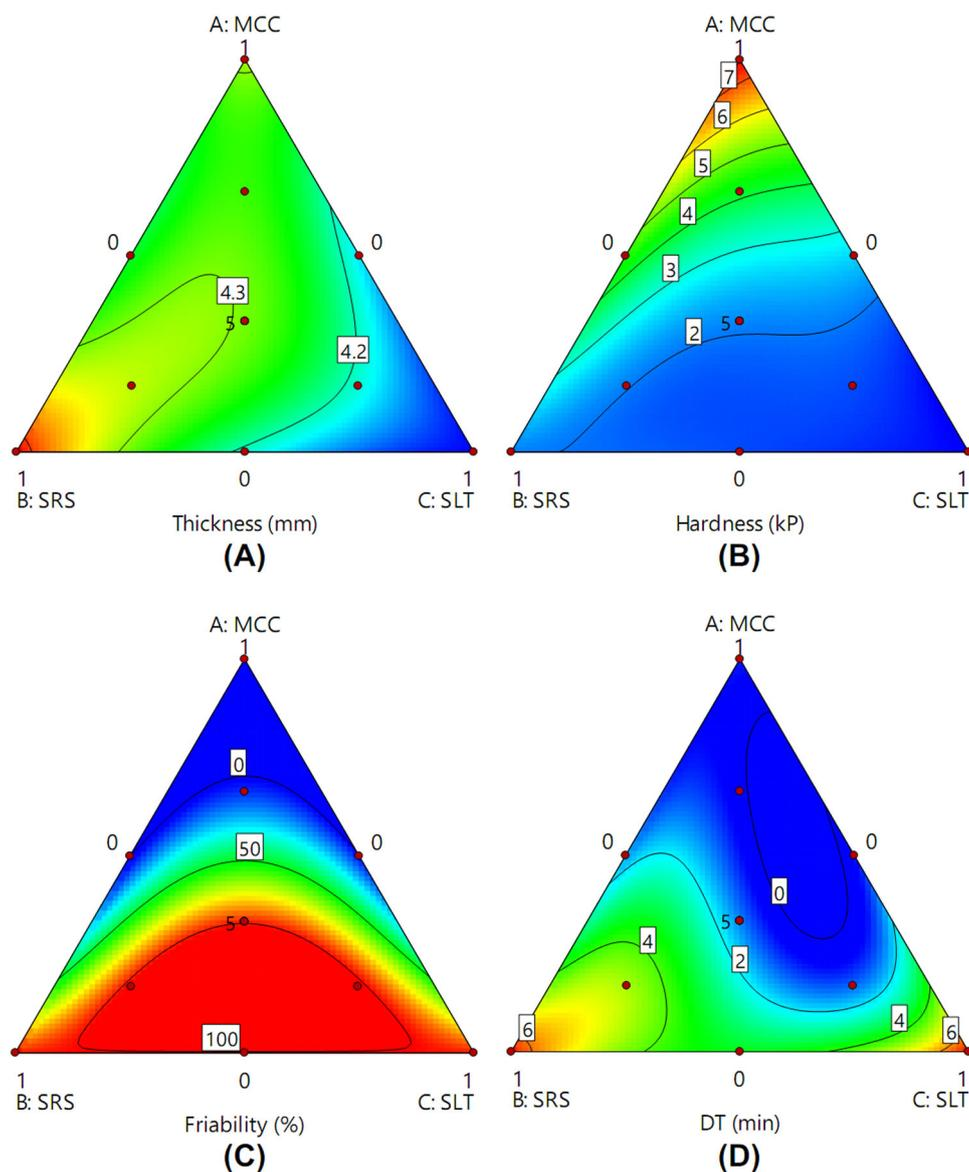
**Figure 1.** Contour plots of (a) thickness, (b) hardness, (c) friability, and (d) disintegration time of *Boesenbergia rotunda* (L.) Mansf. extract tablet obtained from the simplex lattice design.
