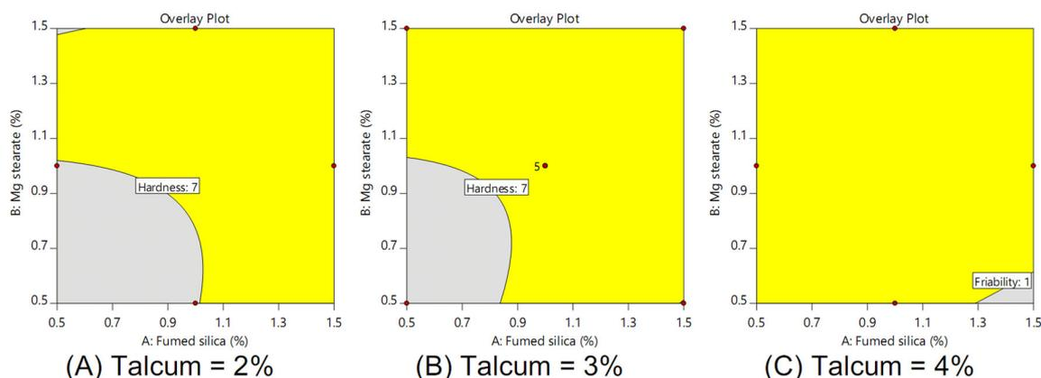
**Figure 3.** Design spaces that *Boesenbergia rotunda* (L.) Mansf. extract tablet had hardness of 5–7 kP, friability of less than 1%, and disintegration time of less than 1 min at different talcum levels: (a) talcum 2%, (b) talcum 3%, and (c) talcum 4%.
