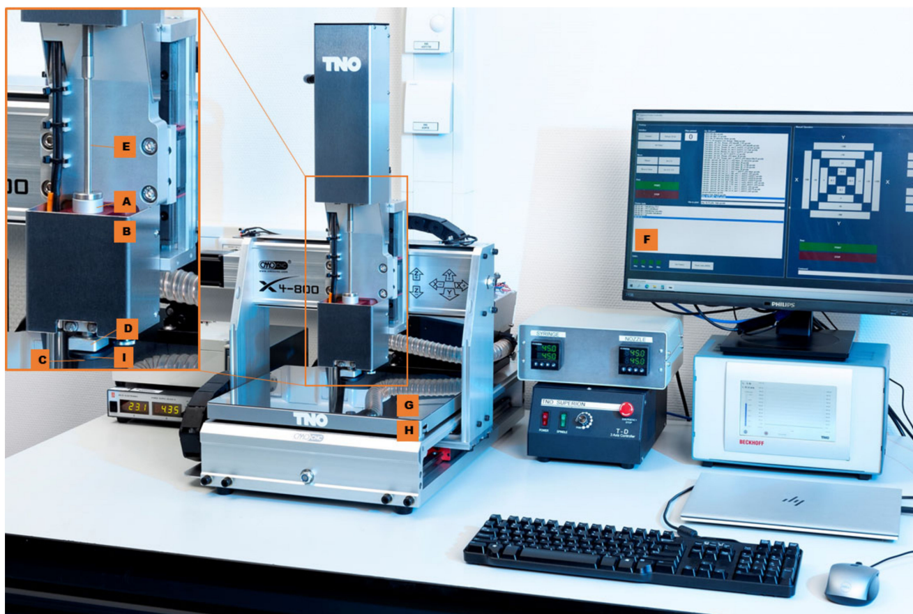
Figure 2. Used printer setup; syringe (A), the heating element of the syringe (B), nozzle (C), the heating element of the nozzle (D), piston (E), computer with Pronterface (F), printing platform (G), heating bed (H), and cooling (I).
