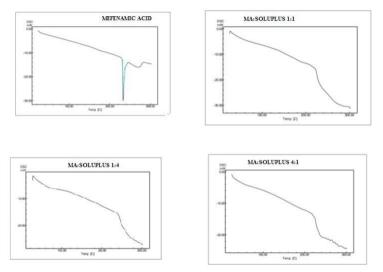
Figure 2. DSC thermograms of MA, MA: Soluplus (1:1,1:4 and 4:1)
