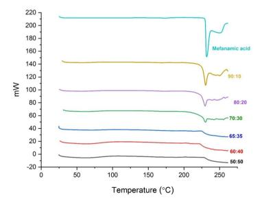
Figure 1. Thermograms of the MA-Soluplus physical mixtures (% w/w)
