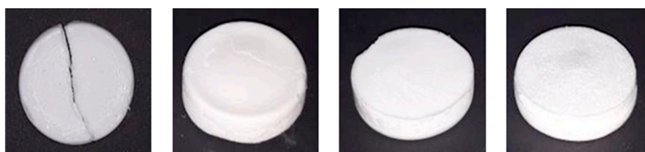
Fig. 1. Appearance of oral lyophilizates obtained from pre-lyophilized liquid formulation with 6% (w/w) of excipients in the mass ratios gelatin:PVP K25:mannitol = 0.5:1:5 (F1); 0.5:2:5 (F2); 1:1:5 (F3) and 1:2:5 (F4) (left to right).
