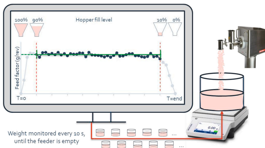
Fig. 1. Graphical representation of the feeder set-up. Discharged excipients are collected in a bin and weighted every 10 s. The feed factor is calculated as the average throughput per revolution between 90% and 10% hopper fill levels.
