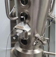
The OseeT probe can be used to measure physical dimensions of film-coatings in both pan coated tablets (Picture Credit: L.B. Bohle Maschinen + Verfahren GmbH) and pellets in fluid beds (Picture Credit: GLATT Process Technology)
