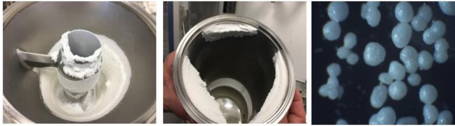
Figure 2. Outcomes from a conventional FBC process whereby Cellets® 100 (median diameter \approx 150 \mu\text{m} ) were coated with a benchtop Würster coater (Mini-Glatt®) using an aqueous polymer dispersion. Shows significant micropellet aggregation in the 'down flow bed' (left), drying zone (centre) and micropellet agglomeration (right).
