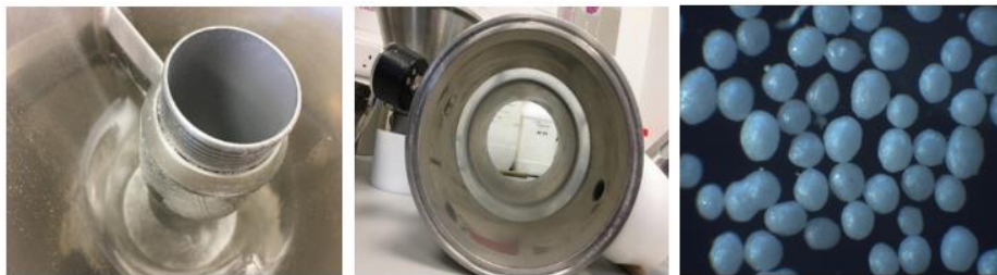
Figure 3. Outcomes from a FBC process following the implementation of the MicroCoat™ technology whereby Cellets® 100 (median diameter \approx 150 \mu\text{m} ) were coated with a benchtop Würster coater (Mini-Glatt®) using an aqueous polymer dispersion. Shows no micropellet aggregation in the coating chamber and non-agglomerated micropellets after coating was completed.
