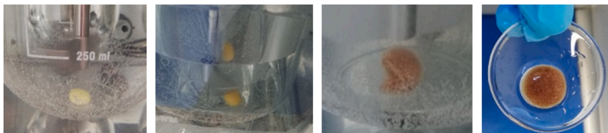
Fig. 6. Appearance of the F1 drugmies during the 2 h gastro-resistance test: starting with the image on the right, the drugmies at 0 min, 15 min, 30 min and 120 min are shown.
