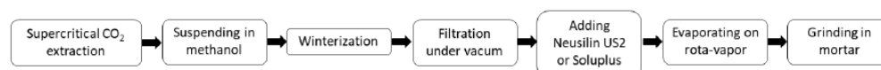
Figure 2. Scheme of preparation of co-dispersion delivery systems of Henola inflorescences extract with Neusilin US2 and Soluplus.
