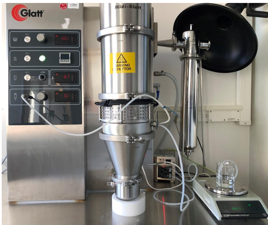
Figure 3.1. Fluid bed granulation set up.
