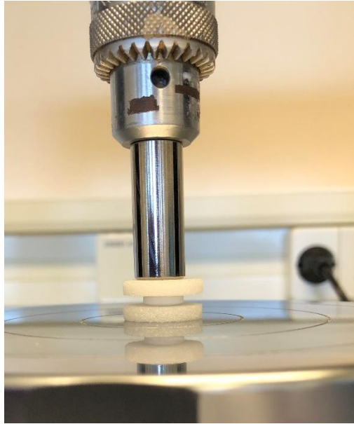
Figure 4.20. Set up of the texture analyzer with filters above and under the tablet and a probe applying and measuring the force on the ODT.
