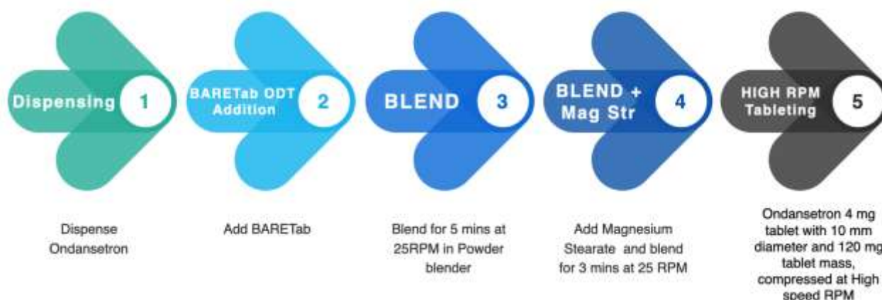
Figure 2: Ondansetron tablet preparation flow chart
