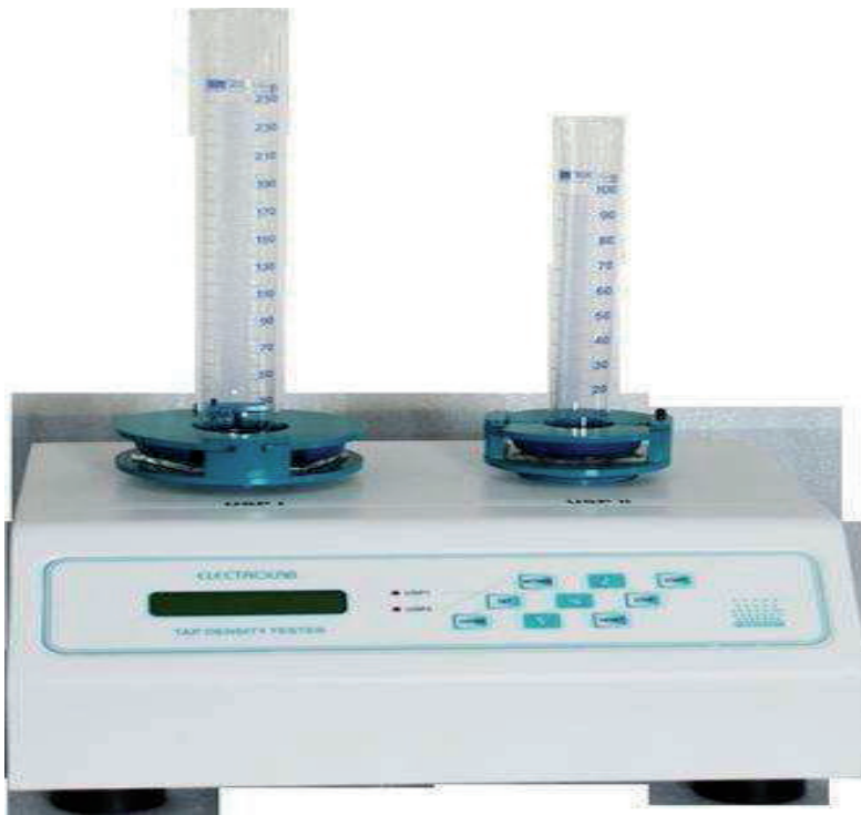
Fig.3 Tapped density tester
