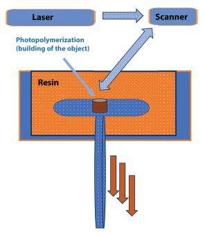
Figure 4. 3D Printing by Photopolymerization (SLA).
