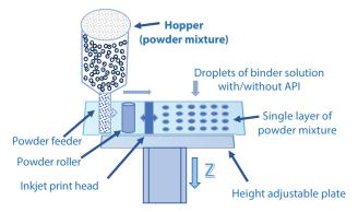
Figure 3. Powder-Based 3D printing.
