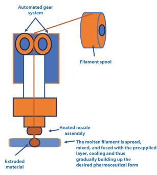
Figure 5. 3D printing by extrusion (FDM).
