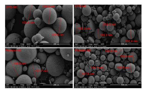
**Figure 3.** SEM images of medicated and unmedicated nanoemulsions (optimal formulation). The images on the right depict  $2500 \times$  magnification; the images on the left depict  $100 \times$  magnification.
