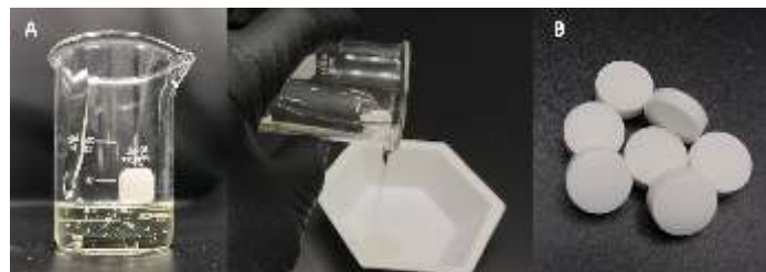
Fig. 1A Vitamin E, Fig. 1B Tablets Made with PROSOLV® 730 and 67 mg (100 IU) of Vitamin E
