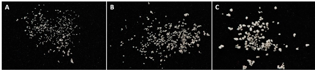
Figure 2. The image of freeze-dried microspheres produced using (A) 150 \mu\text{m} , (B) 300 \mu\text{m} , (C) and 450 \mu\text{m} nozzle sizes.
