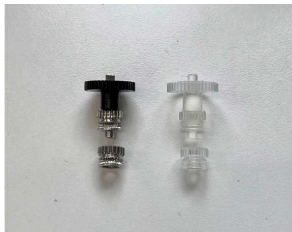
Fig. 10. The original (left-hand side) and the customised extrusion gear set with smaller gear teeth (right-hand side). The custom extrusion gear set was 3D printed and modified from the original design to help improve printability.
