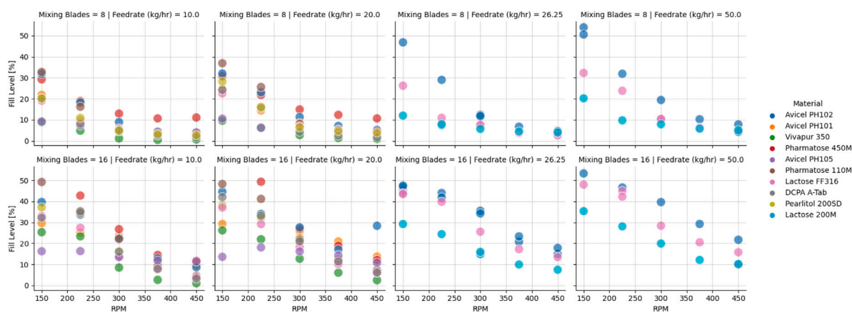
Fig. 11. Scatter graphs showing the fill level response of the materials used for the experiment with respect to the three processing parameters: RPM, Mixing Blades, and Feedrate (kg/h).
